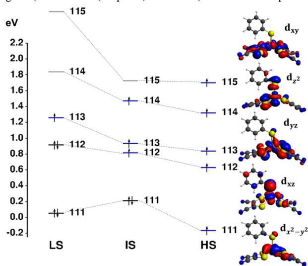
Figure 4. Calculated Fe 3d orbital splitting of complex **1** in the  $S=1/2$  (LS),  $S=3/2$  (IS) and  $S=5/2$  (HS) states. Doubly occupied orbitals are shown in black, singly occupied in blue and unoccupied in grey.
