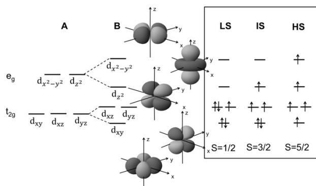
Figure 2. Crystal field splitting of the 3d orbitals in **A**) an octahedral system and **B**) a penta-coordinate square-pyramidal complex. For iron(III) the 3d<sup>5</sup> electron occupancies are shown for the low-spin (LS) S=1/2 state, the intermediate-spin (IS) S=3/2 state, and the high-spin (HS) S=5/2 state.
