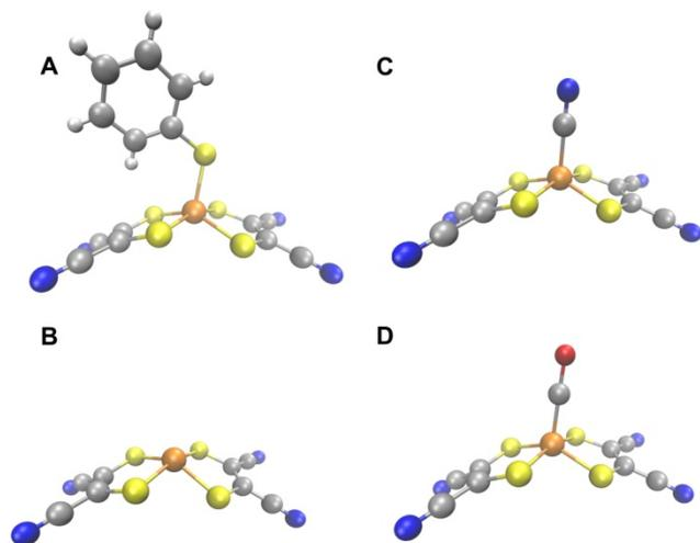
Figure 9. A) Complex **1**, B) vacant axial site (complex **2**), or axial ligand substitution by C) a cyanide ligand (CN<sup>-</sup>, complex **3**) or D) a carbonyl ligand (CO, complex **4**).
