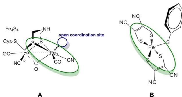
Figure 1. Schematic representation of the [FeFe]-hydrogenase active site (A) and complex **1**, a penta-coordinate Fe(III) functional mimic of hydrogenase<sup>[8]</sup> (B).
